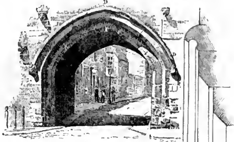
Gate of Close, Salisbury Cathedral, England. D, D. dripstone. (Right-hand figure shows a section of the gateway.)
